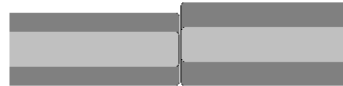
CLADDING DIAMETER MISMATCH
