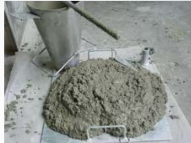
Slump S5 – > 220mm
