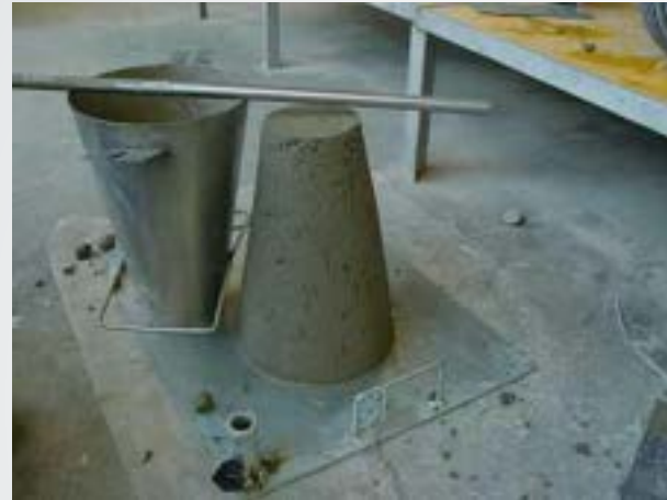
Slump S1 – 0-40mm
