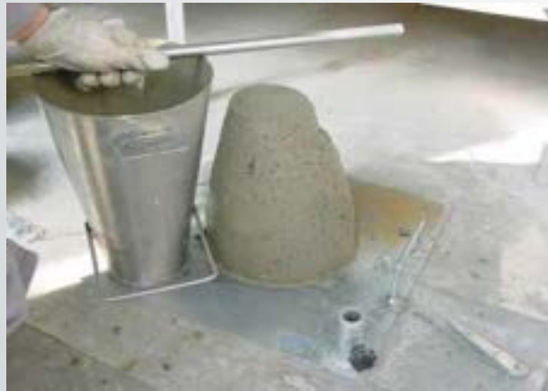
Slump S2 – 50-90mm
