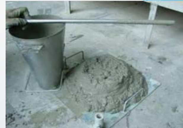
Slump S4 – 160-210mm
