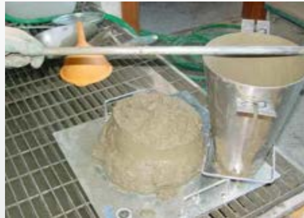
Slump S3 – 100-150mm
