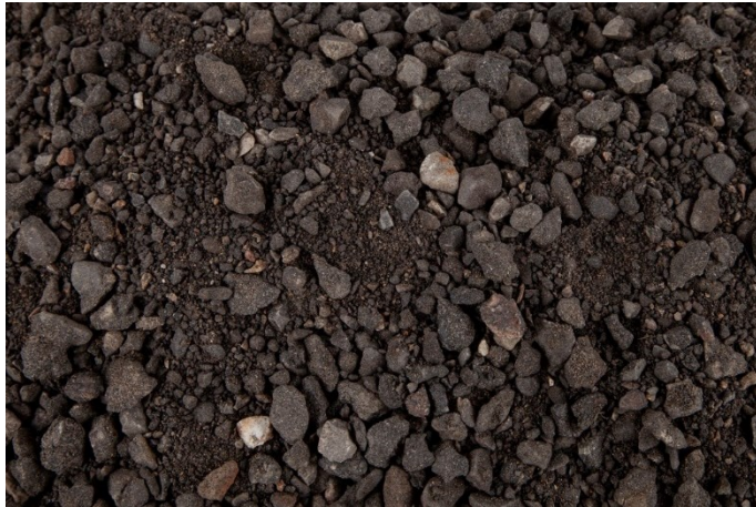
Conglomerato bituminoso fresato
