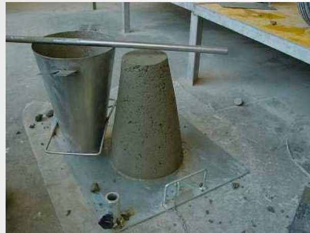
Slump S1 – 0-40mm
