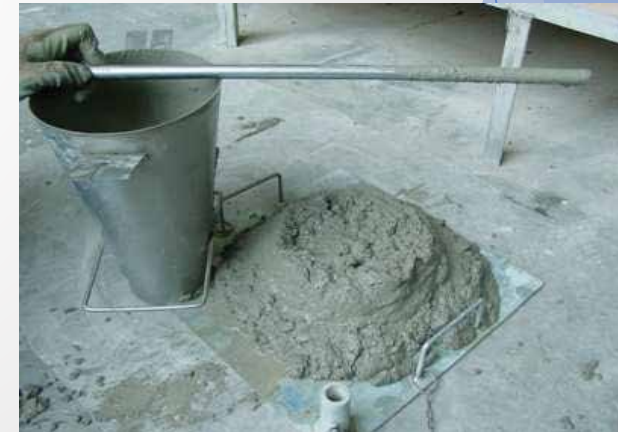
Slump S4 – 160-210mm
