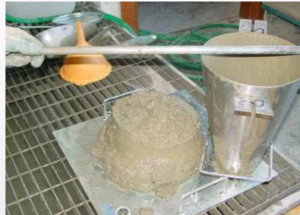
Slump S3 – 100-150mm
