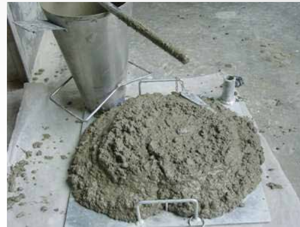
Slump S5 – > 220mm
